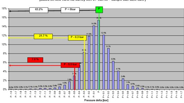
Distribution of tyre pressure per wheel [based on New RDW NL survey Nov 07- Jan 08 - sample size 8250 cars ]
