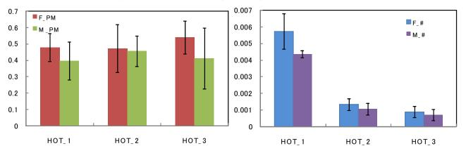
F\_PM : PM by full tunnel, M\_PM : PM by partial tunnel F\_F : number by full tunnel, M\_PM : number by partial flow
