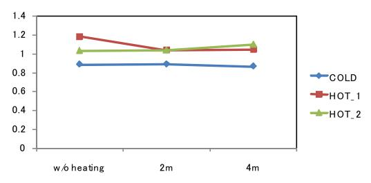
Without heating : length = 0.8m 2m, 4m : heated to 150 degree C
