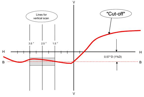
If the "cut-off" complies with the quality requirements of paragraph 2. of this annex, the beam adjustment may be performed instrumentally.
