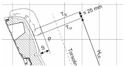
new criteria: measuring of thickness S [25 mm] above lower edge
