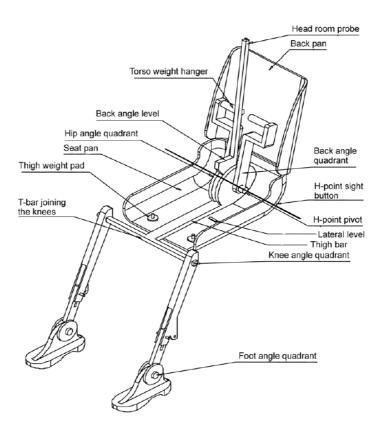
Figure 1 - 3 DH machine elements designation
