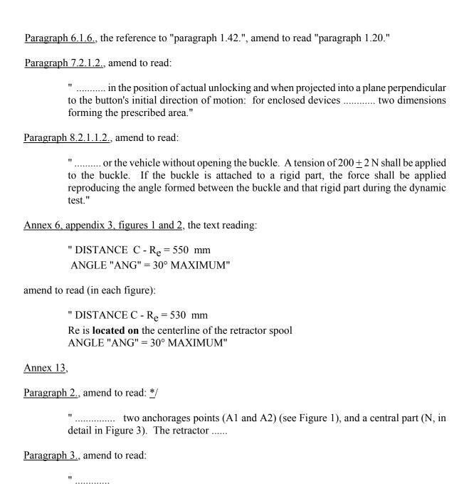
Belt retractor R shall be fitted to trolley anchorage such that the spool centre-line is positioned on Re
