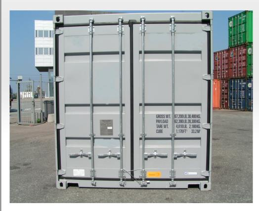
An elongated door handle hub (sometimes referred to as a security hub) that extends at least 25 mm below the rivet hole or pivot point, shall be used on the right hand door to prevent the handle from being removed even if the rivet is removed.
