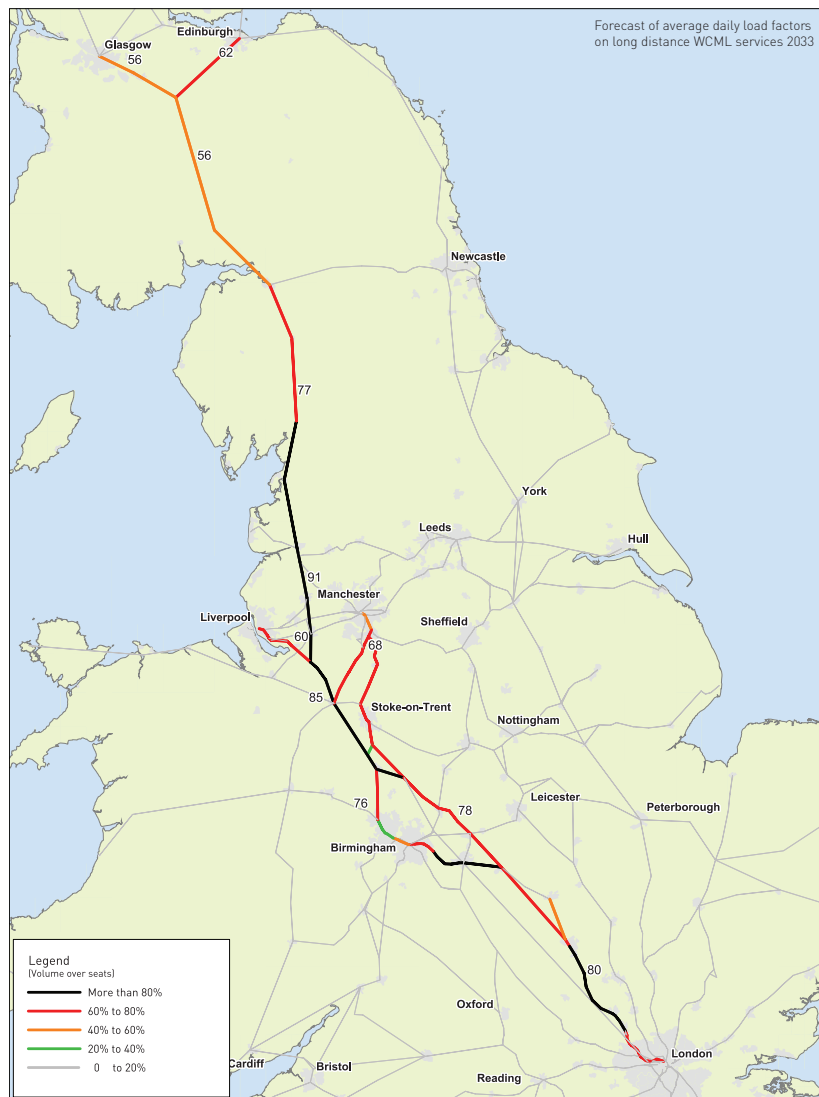
Figure 1.2b Forecast of average daily load factors on long distance WCML services in 2033
