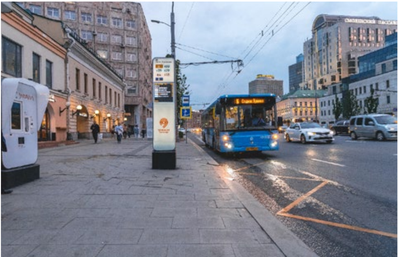
FIGURE 3.13 MOSCOW. THE BUS STOP IS EQUIPPED WITH TICKET MACHINE AND A DISPLAY BOARD WITH ACTUAL ARRIVAL TIME
