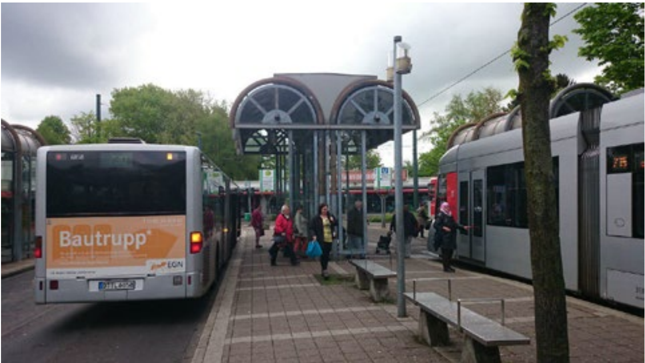
FIGURE 3.16 DÜSSELDORF, GERMANY. CROSS-PLATFORM TRANSFER BETWEEN BUS AND TRAMWAY PROVIDES MOST SAFE AND FAST TRANSFER, ALLOWS TO REMOVE EXCESSIVE ROUTES AND RAISES THE ROUTE NETWORK EFFICIENCY
