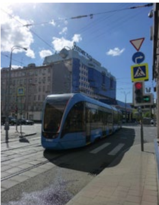
FIGURE 3.50 MOSCOW. IMPLEMENTATION OF PUBLIC TRANSPORT PRIORITY AT THE INTERSECTION: ONLY PUBLIC TRANSPORT ALLOWED TO CROSS THE STREET IN A DIRECT WAY. THE SAME METHOD WAS APPLIED EFFECTIVELY IN TORONTO
