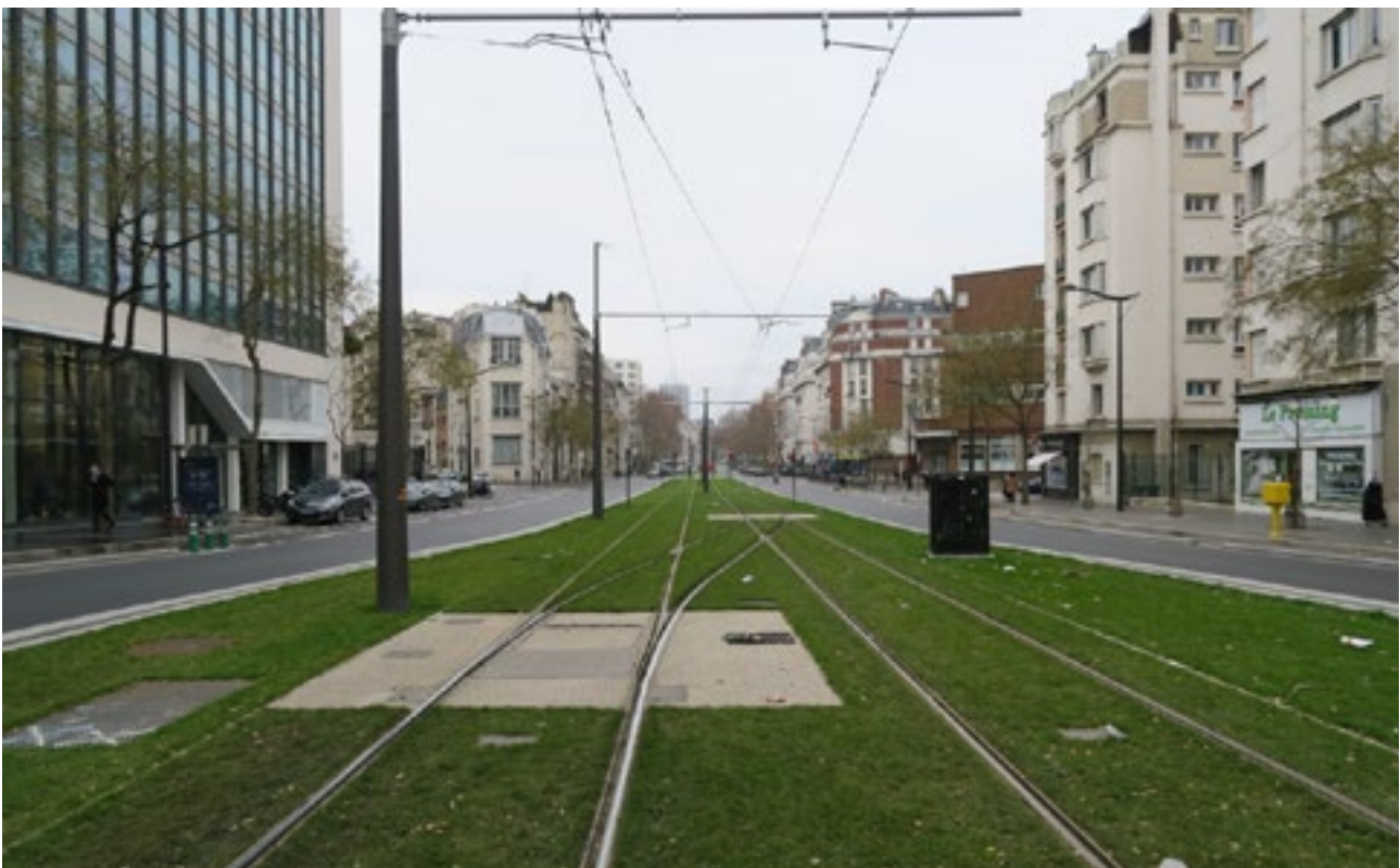
FIGURE 3.48 PARIS. GREEN TRACK IS A TECHNOLOGY, ALLOWING THE EXPANSION OF GREEN SPACE IN THE CITIES
