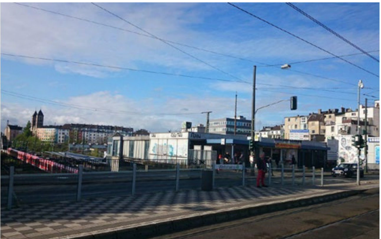
FIGURE 3.27 DÜSSELDORF. TRAMWAY STOP IS PLACED ON THE RAILWAY BRIDGE IN ORDER TO MINIMIZE WALKING DISTANCE AT TRANSFER
