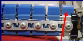
Blue segment face detached - easily re-attached
