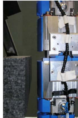
Impact height 0 mm: Centre of knee in line with upper edge of second foam piece
