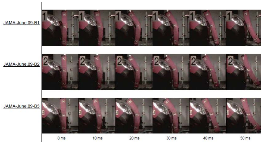
Flex-GTR-prototype JAMA Round Robbing Test Results Kinematics (JAMA-June.09-B1, B2, B3)
