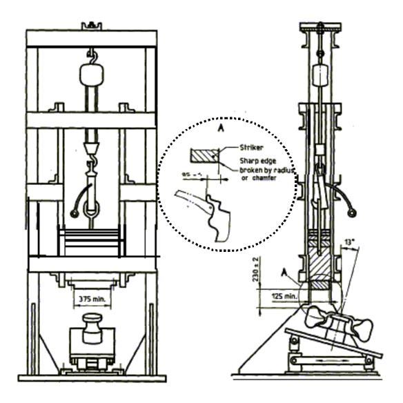
Figure 1 – Impact loading test machine
