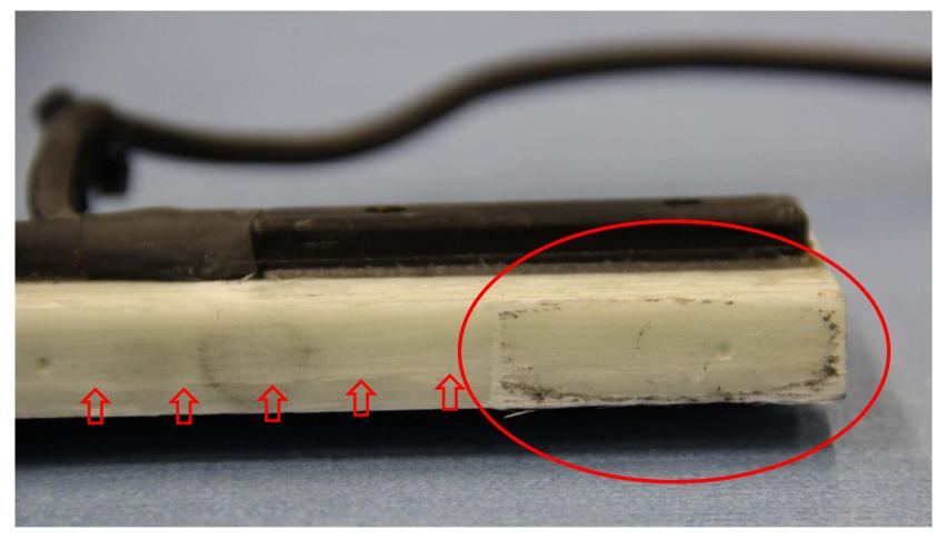
• Wearing and white cracks near/at knee clamping area
