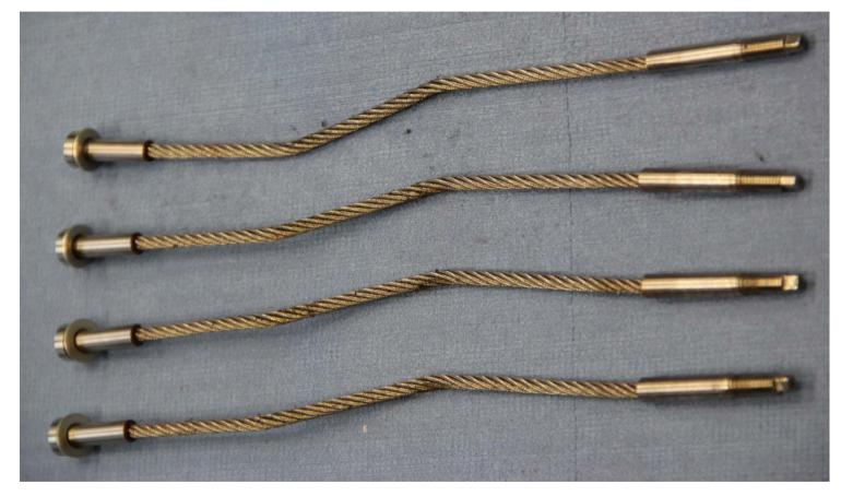
Wearing/deformation at steel cables representing cruciate ligaments
