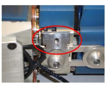
• Stress relief for trigger cable at knee element missing
