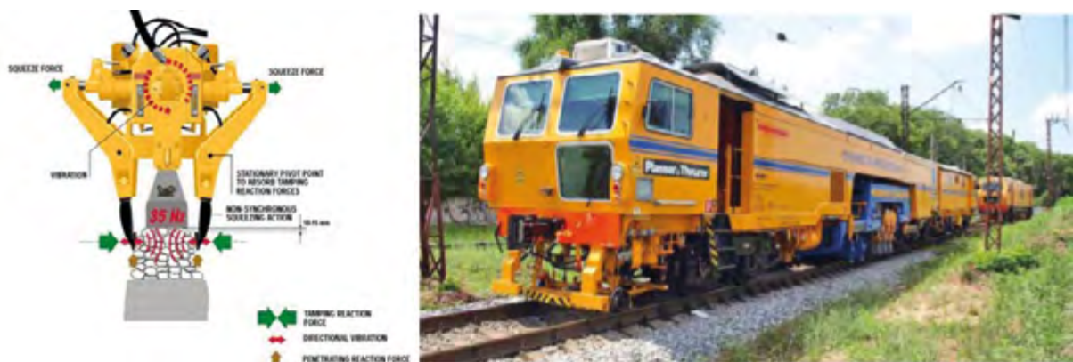
Figure 3.14 - Track tamping machine
