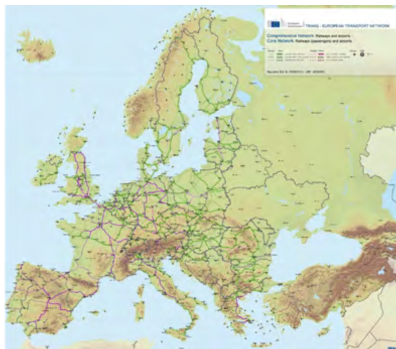
Figure 1.4 - TEN-T core network for railways for passengers (with high-speed links in purple)
