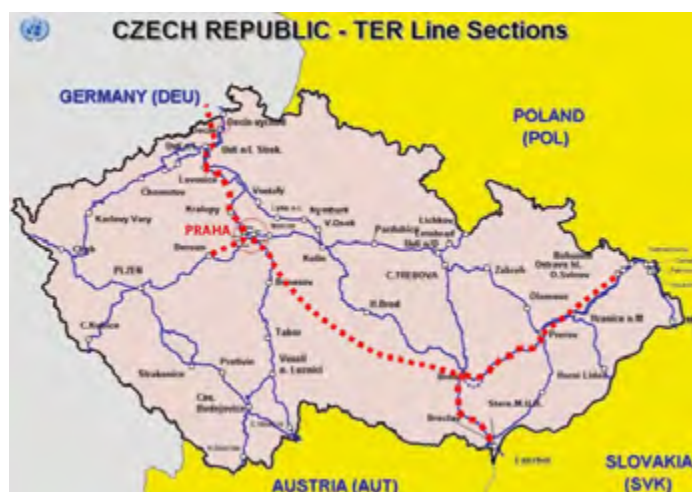
Figure 2.12 - Czech TER network and high-speed projects: Short term: Prague — Lovosice, Brno — Břeclav, Brno — Přerov: bold dotted red lines Long term: Prague — Brno, Lovosice — border CZ-DE, Přerov — Ostrava: dotted red lines
