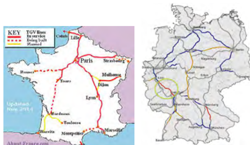
Figure 2.3a and b - High-speed rail networks in France (centre-oriented, a, left) and Germany (networked, b, right)
