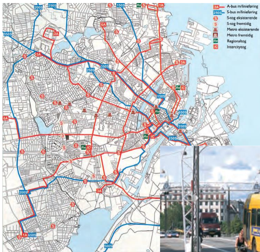
Figure 3.39. The network of main-line A-buses in Copenhagen (Denmark) (red-lined) and suburban express S-buses (blue-lined) complements the network of commuter S-tog trains (S-marked) and metro (M-marked), collectively forming the framework of the Copenhagen public transport with a full tariff integration.
