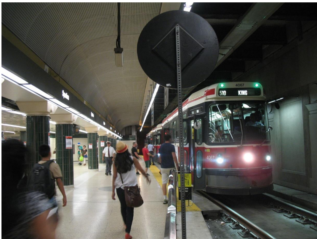
Figure 3.26. Toronto, Canada. Tramway lines are integrated with underground subway stations so as to provide the shortest and comfortable transfer walkways between two rail modes.
