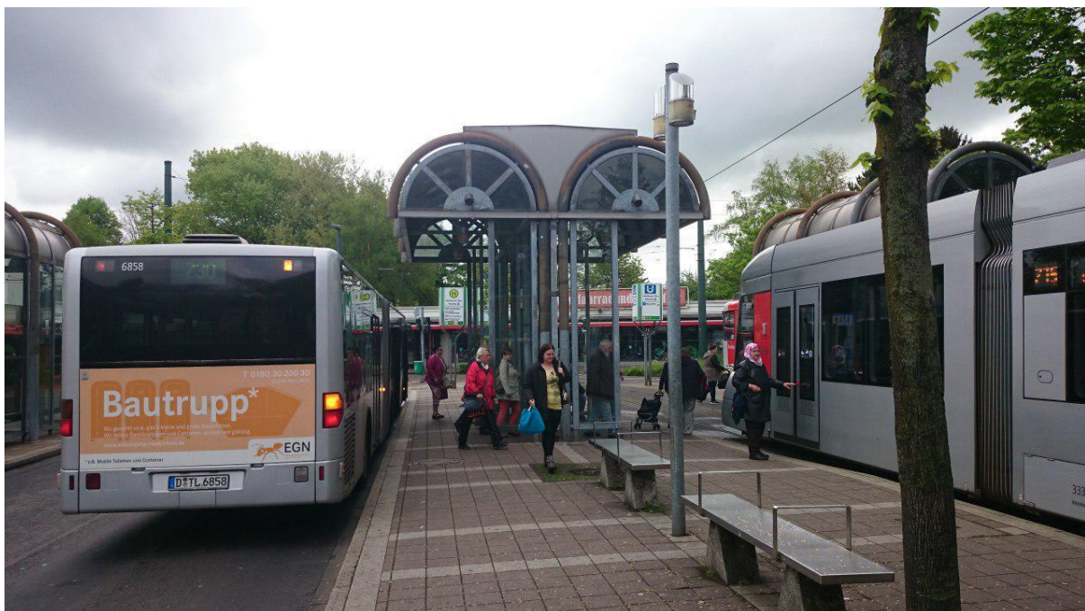
Figure 3.19. Dusseldorf, Germany. Cross-platform transfer between bus and tramway provides most safe and fast transfer, allows to remove excessive routes and rise the route network efficiency
