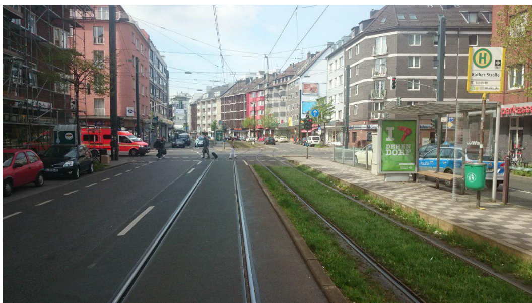
Figure 3.57. Dusseldorf, Germany. Individual solution to separate only one way of tram track in a narrow street conditions.
