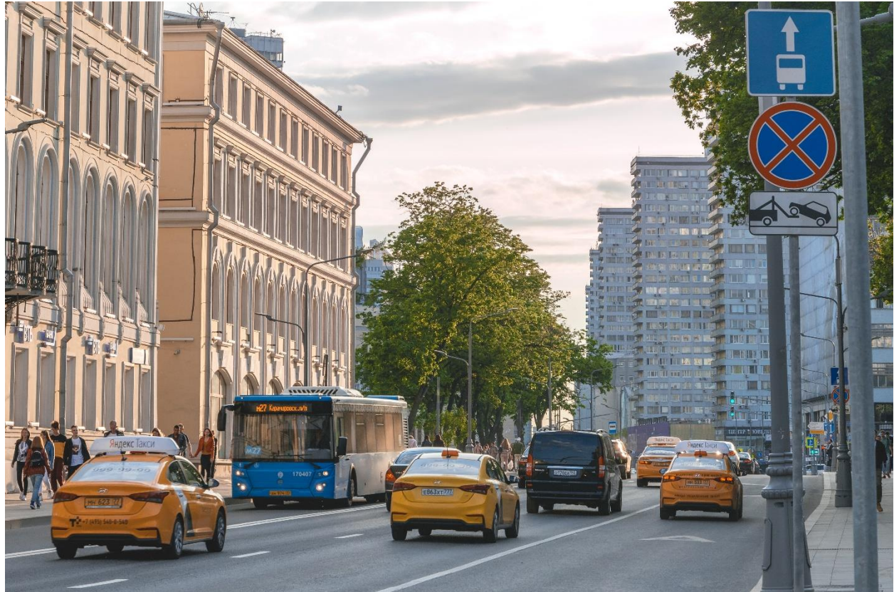
Figure 3.62. Moscow, Russia. Bus lanes, implemented in 2018, provided in both directions on a one-way street so as to provide two-way passenger service.
