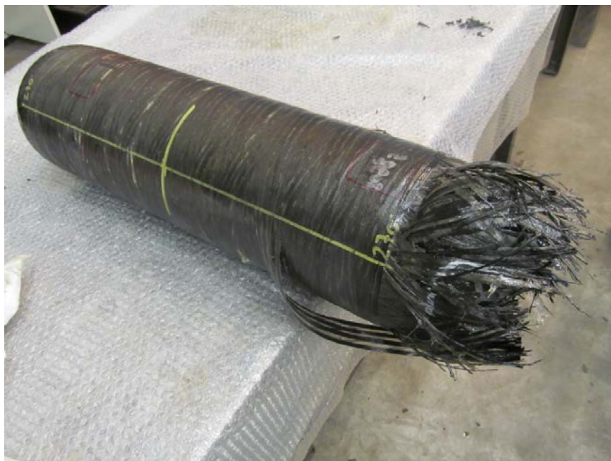
Figure 4-26: Cylinder 10 – Failure location after second fatigue test
