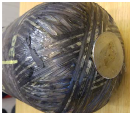
Figure 4-4: Cylinder 2 – Discolored area on capped side
