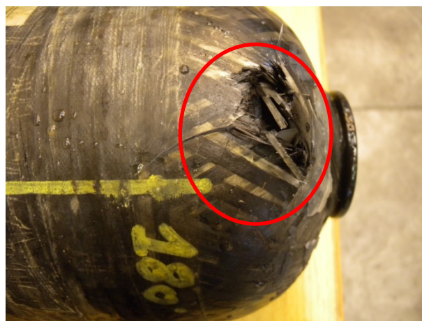
Figure 4-2: Cylinder 1 – Failure location after second hydraulic test
