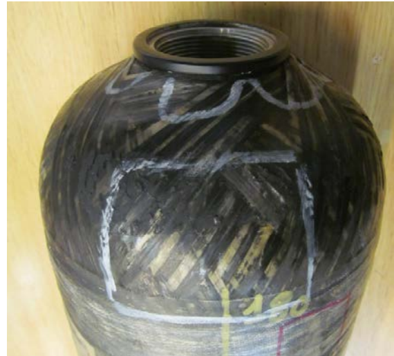
Figure 4-31: Cylinder 12 – Damaged area valve side
