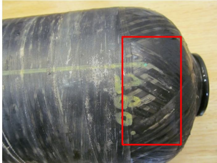
Figure 4-23: Cylinder 10 – Unglued fibers after the first fatigue test
