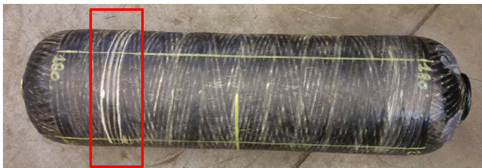
Figure 4-5: Cylinder 2 – Unglued fibers after fatigue test
