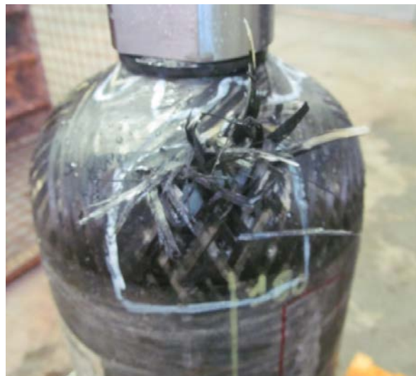
Figure 4-32: Cylinder 12 – Failure location after second hydraulic test
