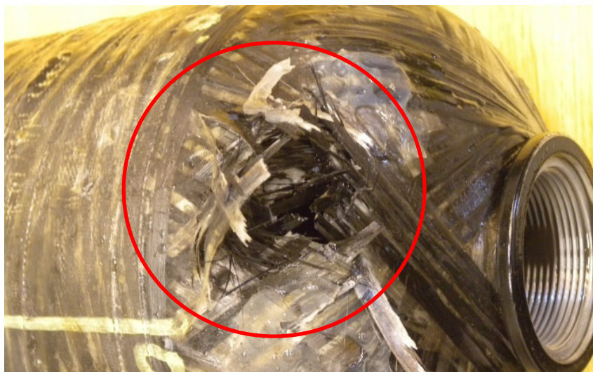
Figure 4-9: Cylinder 4 – Failure location after second hydraulic test
