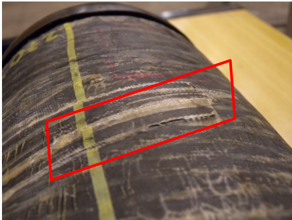
Figure 4-12: Cylinder 6 – Unglued fibers
