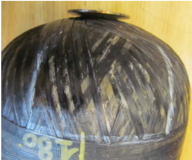
Figure 4-27: Cylinder 11 – Damaged area capped side
