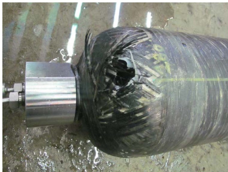
Figure 4-22: Cylinder 9 – Failure location after second hydraulic test
