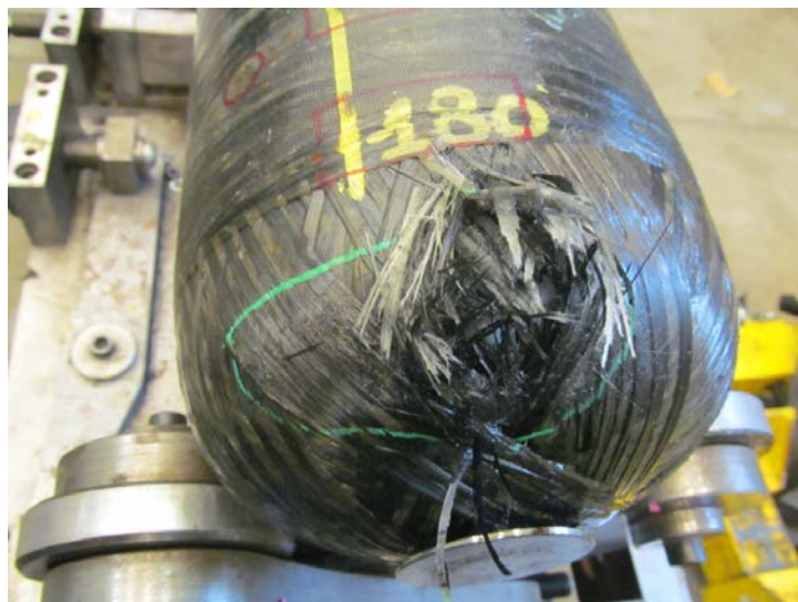
Figure 4-11: Cylinder 5 – Failure location after second fatigue test
