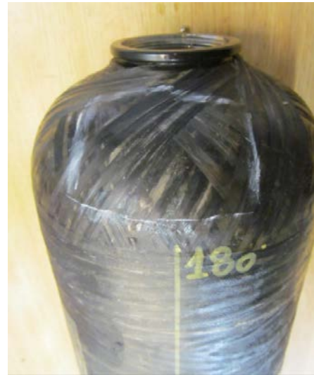
Figure 4-28: Cylinder 11 – Damaged area valve side
