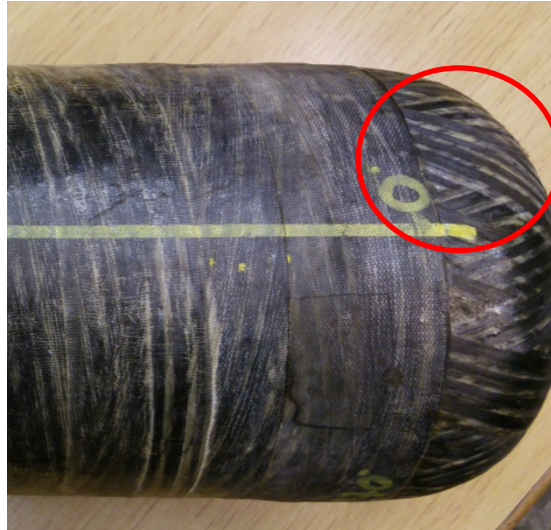
Figure 4-6: Cylinder 3 – Discolored area close to capped side (0°)
