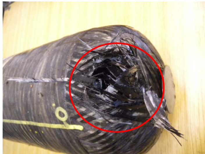
Figure 4-7: Cylinder 3 – Failure location after second hydraulic test
