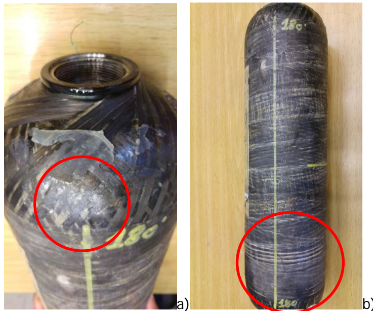
Figure 4-1: Cylinder 1- Main damages before second hydraulic test: a) discolored area; b) detached fibers
