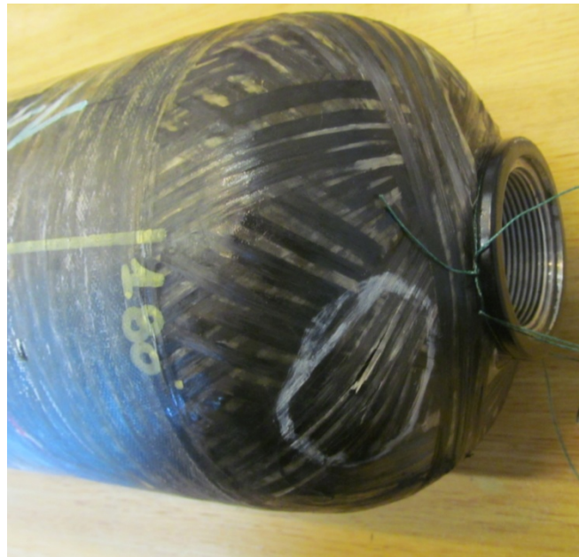
Figure 4-25: Cylinder 10 – Broken fibers on the valve dome
