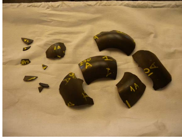
Figure 3-3: Parts of a broken protective dome collected and marked after removal
