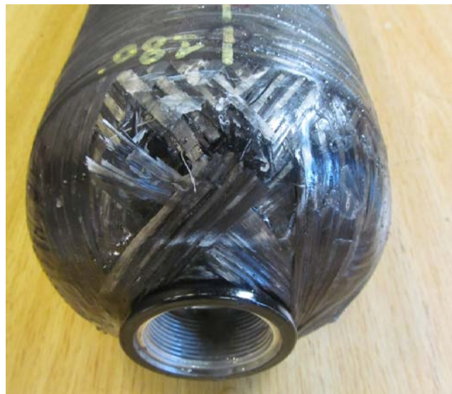
Figure 4-20: Cylinder 8 – Failure location after second hydraulic test
