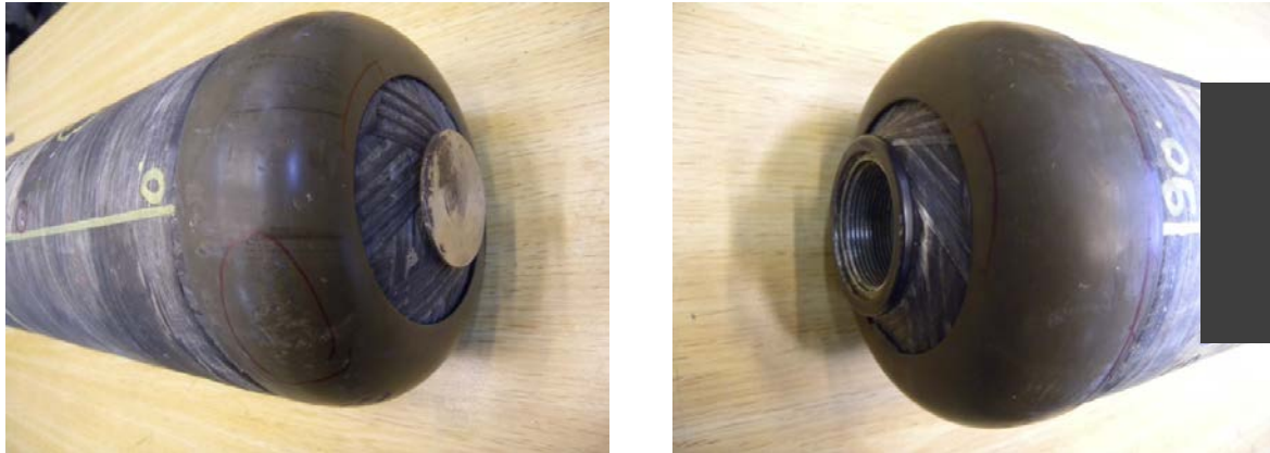
Figure 4-15: Cylinder 7 – Protective domes after the first drop test
