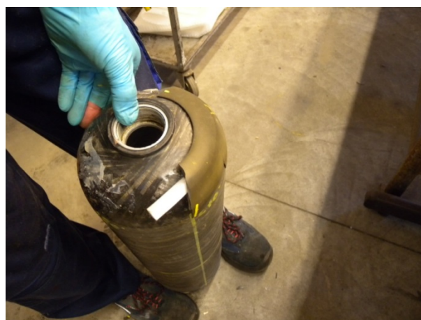
Figure 3-2: Protective dome removal using a PTFE wedge
