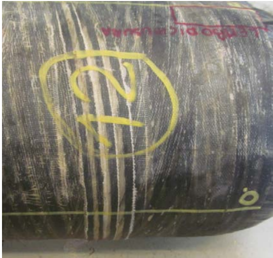
Figure 4-30: Cylinder 12 – Unglued fibers
