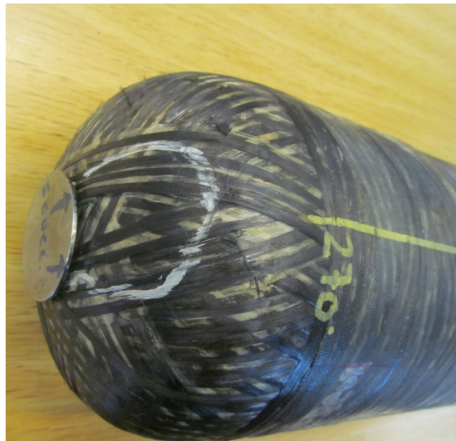
Figure 4-24: Cylinder 10 – Strongly discolored area after drop test
