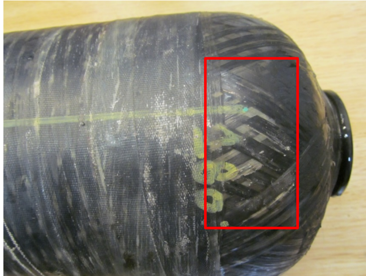
Figure 4-21: Cylinder 9 – Discolored area close to valve capped side (180°)
