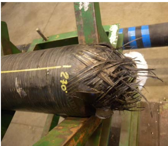
Figure 4-16: Cylinder 7 – Failure after first fatigue test
