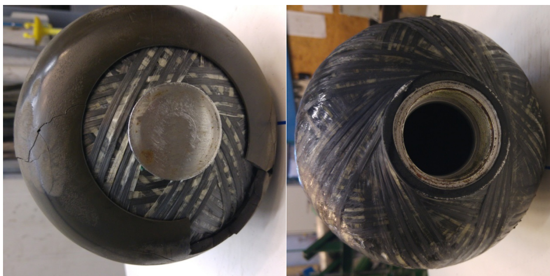
Figure 2-3: Dummy cylinder - Damages on the capped side protective dome after drop tests
