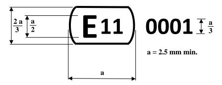
The above approval mark affixed to a filament light source indicates that the light source has been approved in the United Kingdom (E 11) under the approval code 0001."
