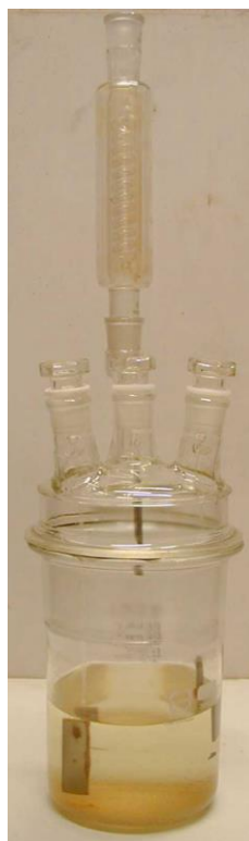
Figure 37.4.2.2: EXPOSURE RECEPTACLE WITH REFLUX CONDENSER
