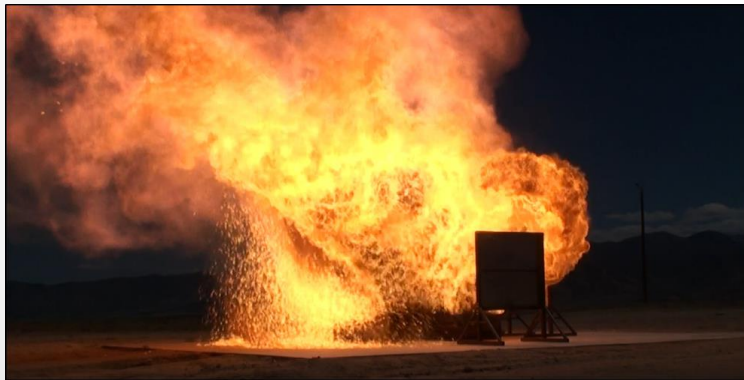
HD 1.3: fire hazard
