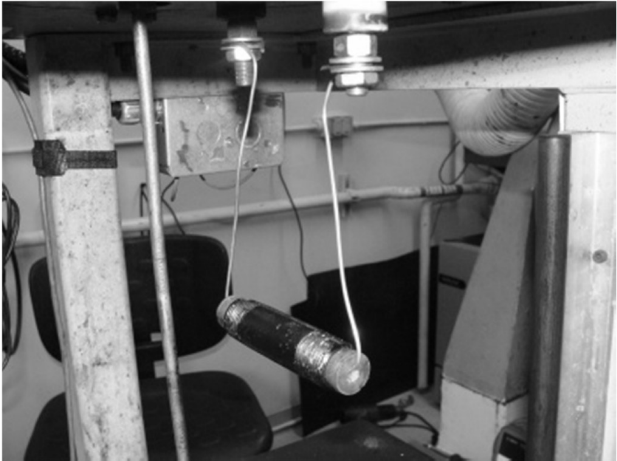
Test cell mounted horizontally under the cover of the pressure vessel (copper conductors connected to vessel's fixed electrodes)
