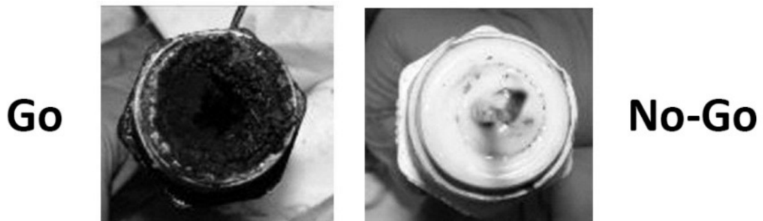
Typical aspect of the test cell after a 'go' (left) and 'no-go' (right) event
