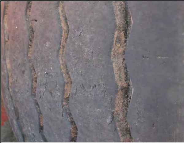
Figure 68: Abrasions on the tyre treads of tyre 2D.
