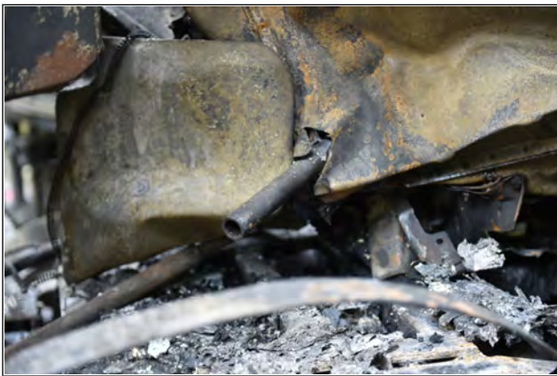
Figure 65: Close-up view, from the rear of the tractor unit, of the metal rod that passed through the rear wall of the cab
