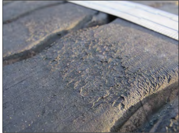
Figure 69: Abrasions on the treads of tyre 1D
