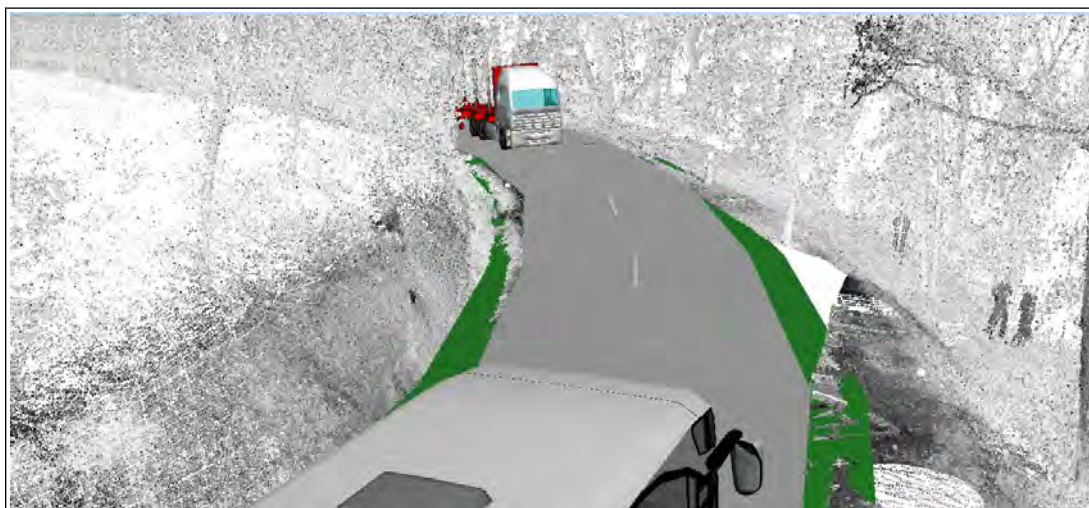
Figure 74: Position of the vehicles at t = 4.50 s, at the moment when the coach driver first saw the articulated lorry.
