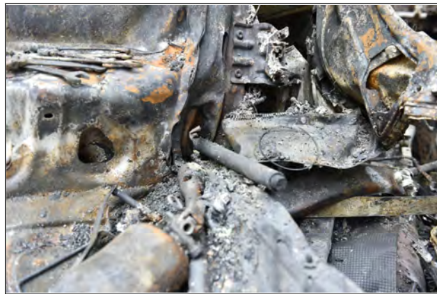
Figure 66: Close-up view, from the front of the tractor unit, of the metal rod that passed through the rear wall of the cab.
