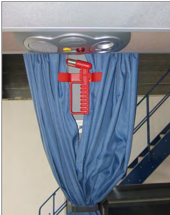
Figure 26: View of an emergency hammer for a side window on a coach similar to the one involved in the accident
