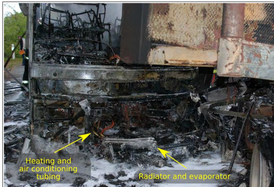
Figure 81: View of the front face of the accident-damaged coach
