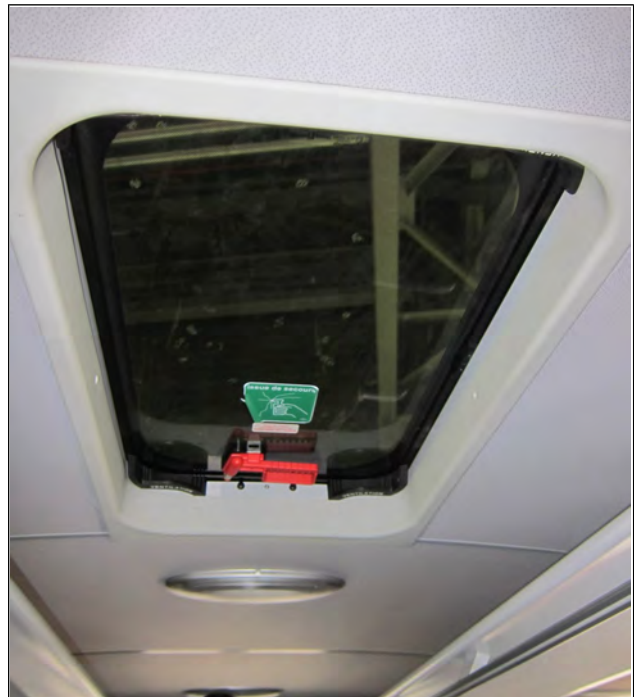
Figure 27: View of an emergency exit on the roof of a coach similar to the one involved in the accident
