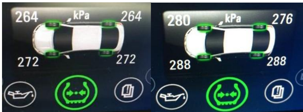
Figure 9. Illustration of a direct TPMS with on board monitoring of all tyres. Left when tyres are cold and right when they are warm (after 100 km). Note: the tyre pressure is given in kPa (280 kPa=2,8 bar) (Photo Erik Roelofsen)
