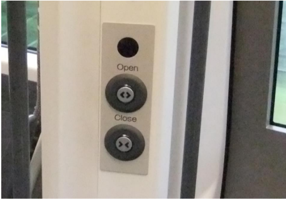
Figure B.4 — Example door control panel with tactile pushbuttons
