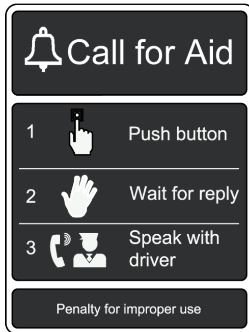
Figure K.9 — Example of alarm or call for aid device functional instructions sign
