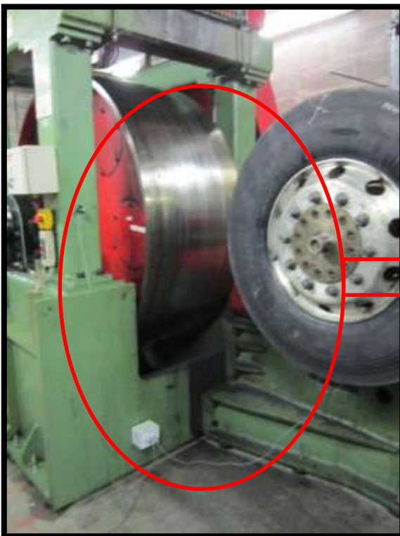
Example of tires (C2 & C3) fitting on HAWITEC-UTAC Load/speed machine and Data Logger NAMI-357
