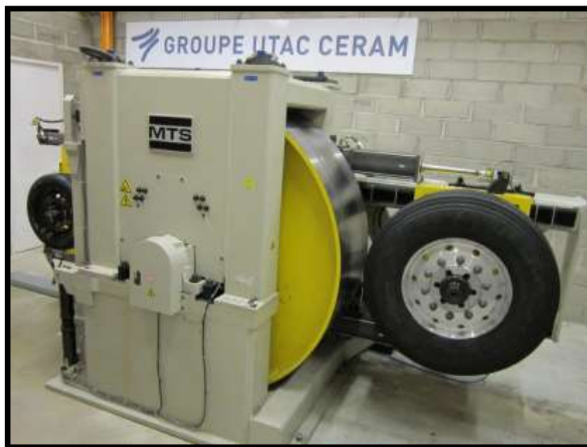
Example of tires (C2 & C3) fitting on MTS-UTAC rolling resistance machine
