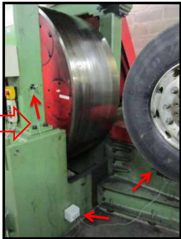
Example of tires (C2 & C3) fitting on HAWITEC-UTAC Load/speed machine and Data Logger NAMI-357
