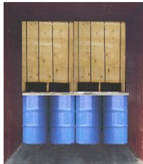
Figure 7.27 Mixed stow, dry over wet goods
