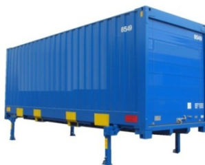
Figure 5.6 Swap body landed on support legs
