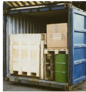
Figure 7.28 Mixed stow, use of pallets
