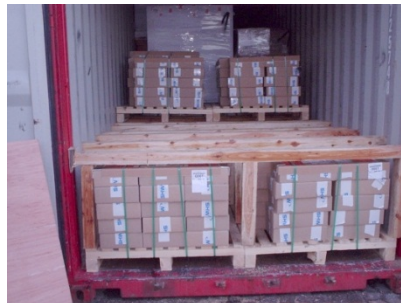
Figure 7.2 Timber temporary floor
