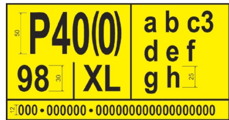
Figure 4.5 Yellow operational mark for trailers
