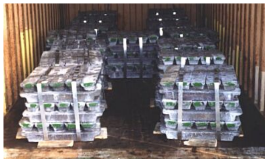
Figure 7.19 Metal ingots unitized by steel banding (securing not completed)
