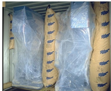
Figure 7.10 Irregular shaped packages blocked with dunnage bags
