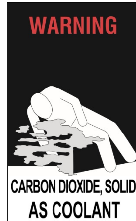
Figure 5.19 Dangerous atmosphere label
