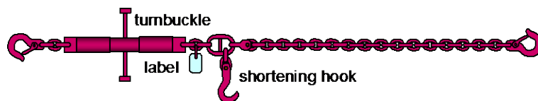
Figure 7.18 Standard chain lashing with shortening hook
