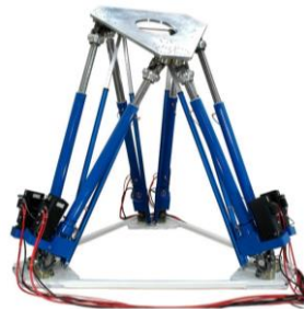
Figure 4: Picture of the 6 degree of freedom test rig
