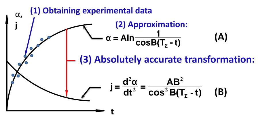
So it is enough to record in discrete form function  $\alpha_i$ =f(t) then approximate it by formula (A) and take a result in form of (B). This is simple. This is accurate.  $\sigma$ <0.03% , R<sup>2</sup> >0.999.
