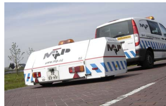
figure 4 cpx measurement of the surface
