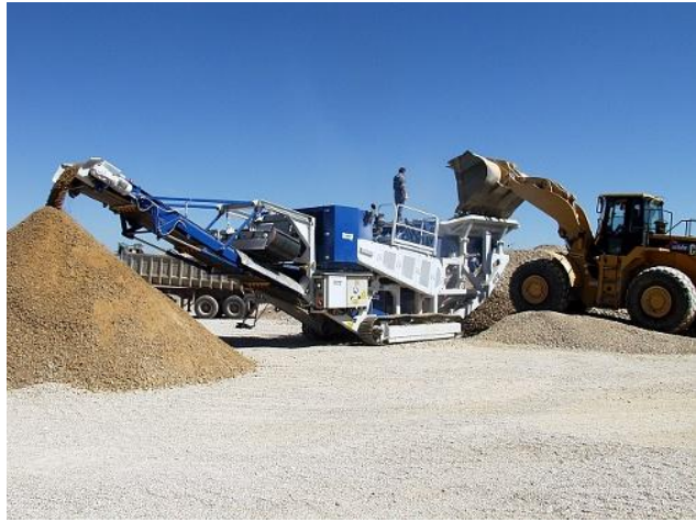
Mobile crusher in operation
