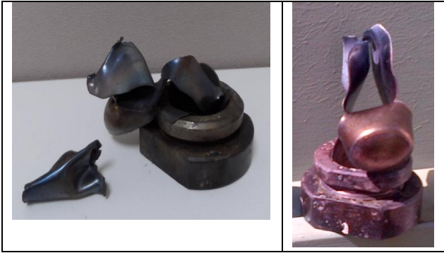
“F”: Tube fragmented into three or more mainly large pieces which in some cases may be connected with each other by a narrow strip;
