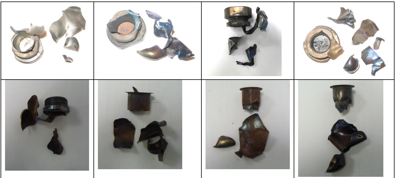
“G”: Tube fragmented into many mainly smaller pieces, closing device undamaged
