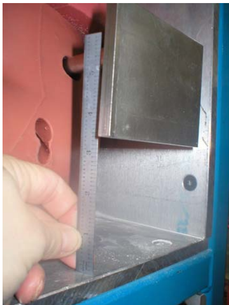
Figure 4. Measuring the H-Point height (left side)
