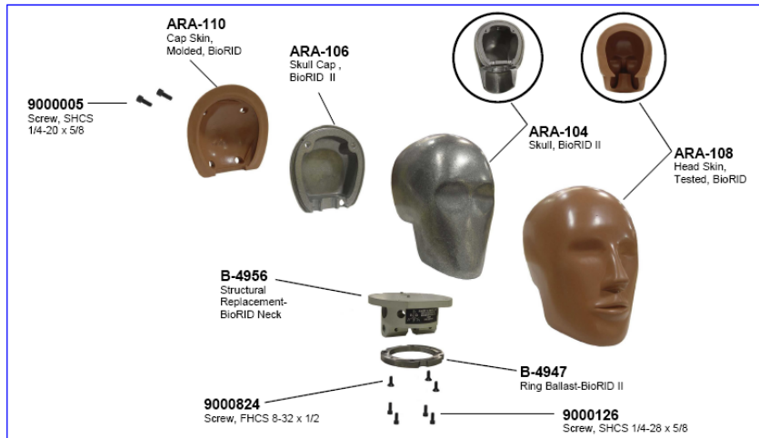
Figure 1. Head assembly exploded view
