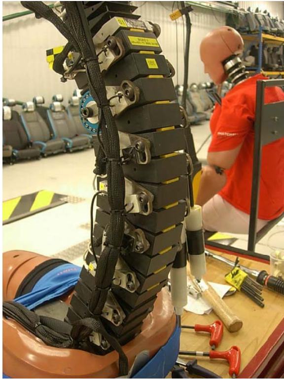
Figure 74 Thoracic Spine cable routing
