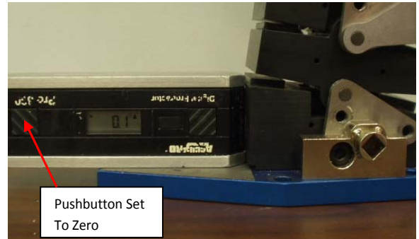
Figure 44 Zero Digital Inclinometer
