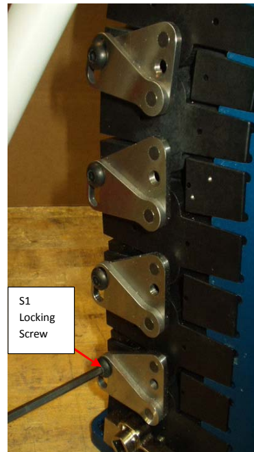
Figure 36. Tighten locking screws
