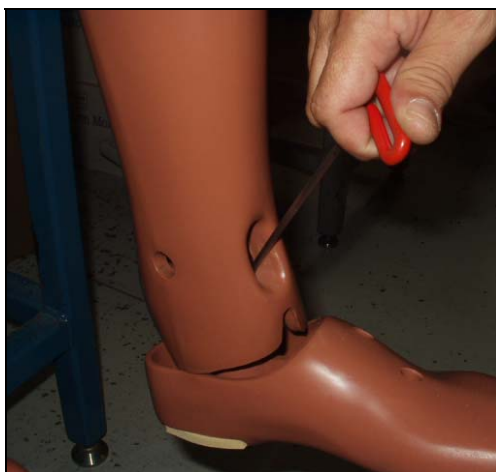
Figure 68 Ankle joint setting
