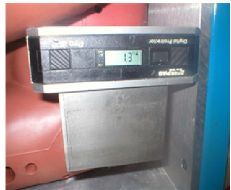
Figure 5. Measuring the H-point tool angle
