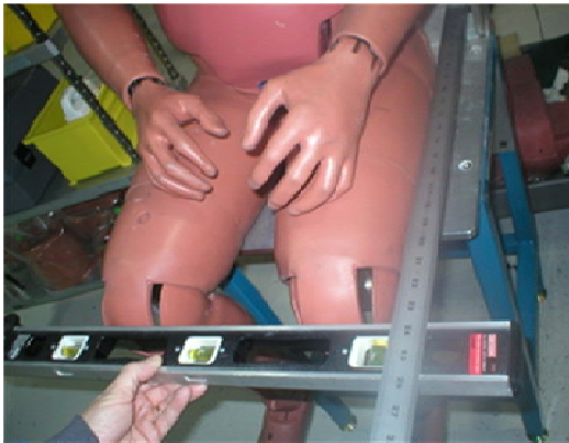
Figure 8. Measuring the knee to buttock length
