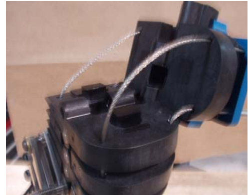
Figure 77 Remove pin and separate vertebra
