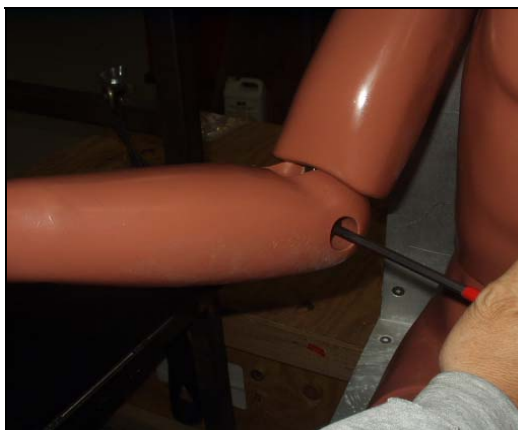
Figure 64 Adjusting the elbow pivot bolt
