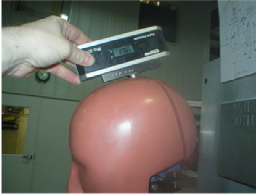
Figure 6. Measuring the angle of the head levelling tool
