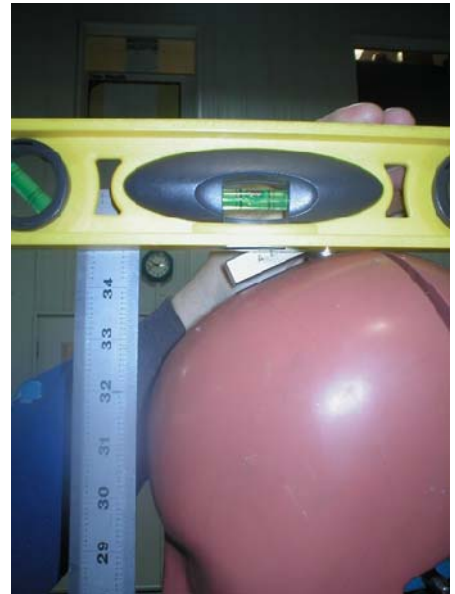
Figure 9 Measuring the seated height of the dummy
