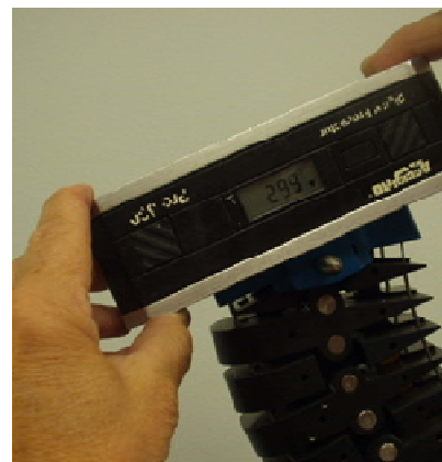
Figure 53 OC Plate angle setting
