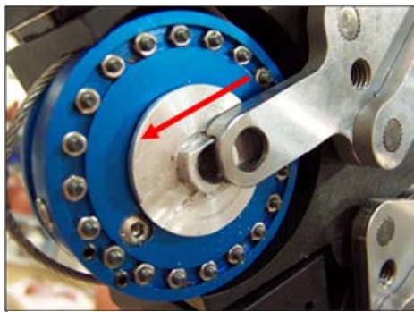
Figure 31 View of Correct Cable Overlap
