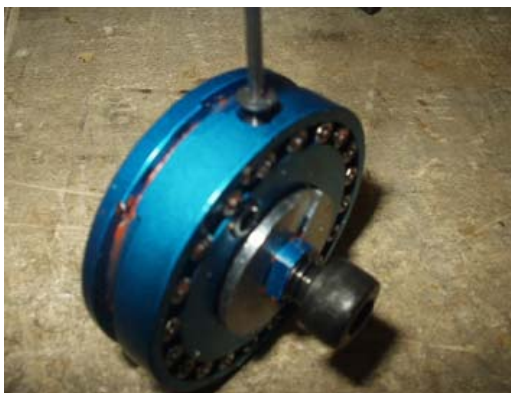
Figure 33. Remove Oil Fill Screw
