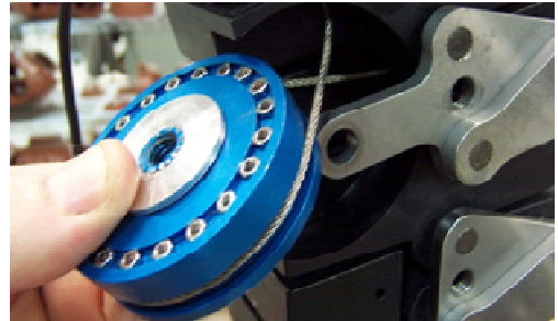
Figure 30 Turn Damper and Disengage Cable
