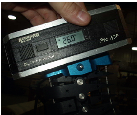
Figure 47 Tilt OC Plate down at the back
