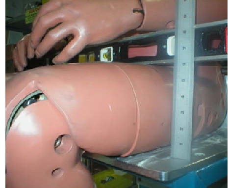
Figure 7. Measuring the thigh clearance
