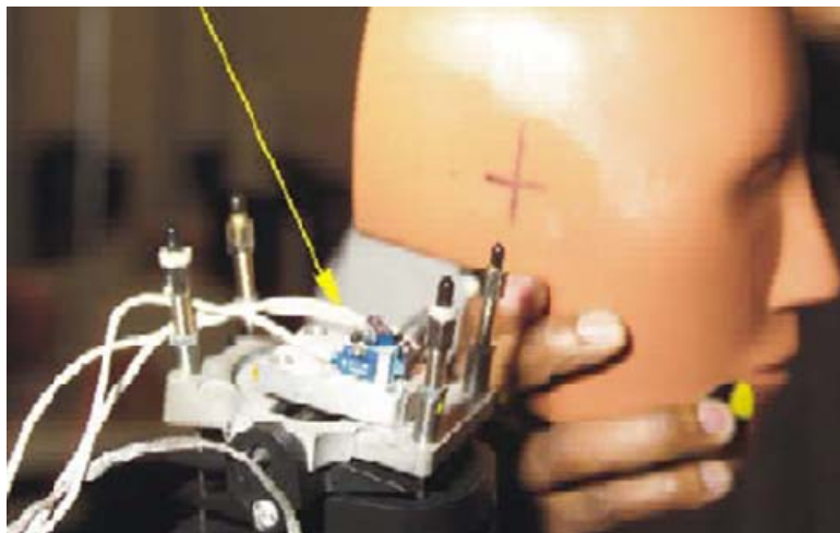
Figure 69 Head accelerometer orientation
