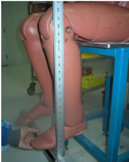
Figure 10 Measuring the left knee pivot height
