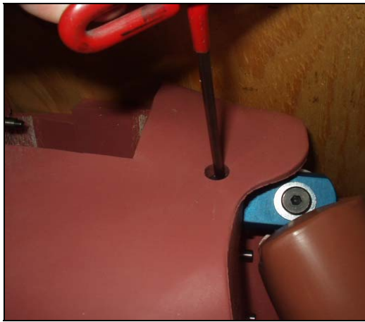
Figure 62 Shoulder joint setting
