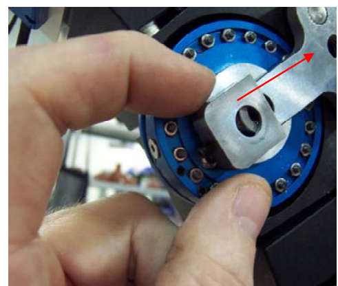
Figure 12 Install Damper Clamp Bracket
