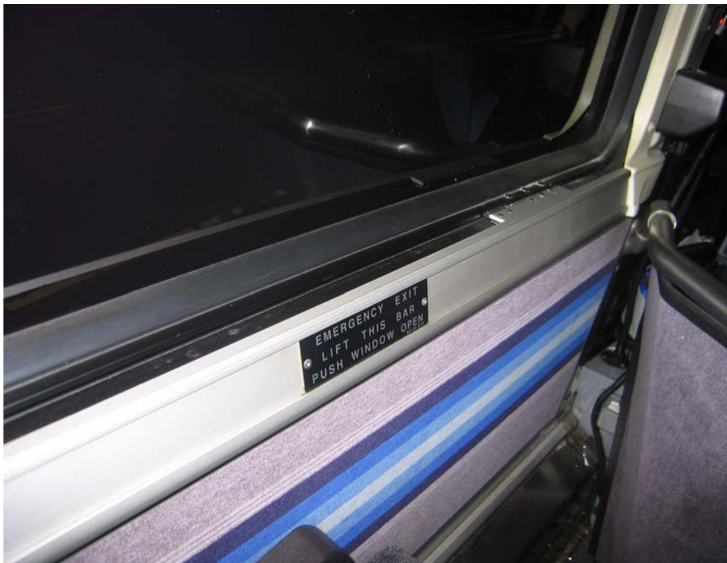
Push out type emergency window (It is locked from inside)
