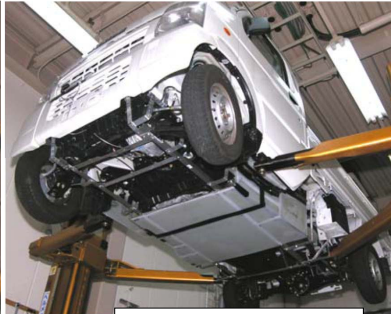
full cover for engine & T/M (under view)
