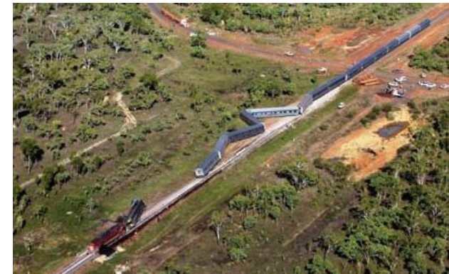
Ban Springs 2006: Trailer road train/Passenger train collision (cause driver behaviour and large heavy road vehicles start/stop time)
