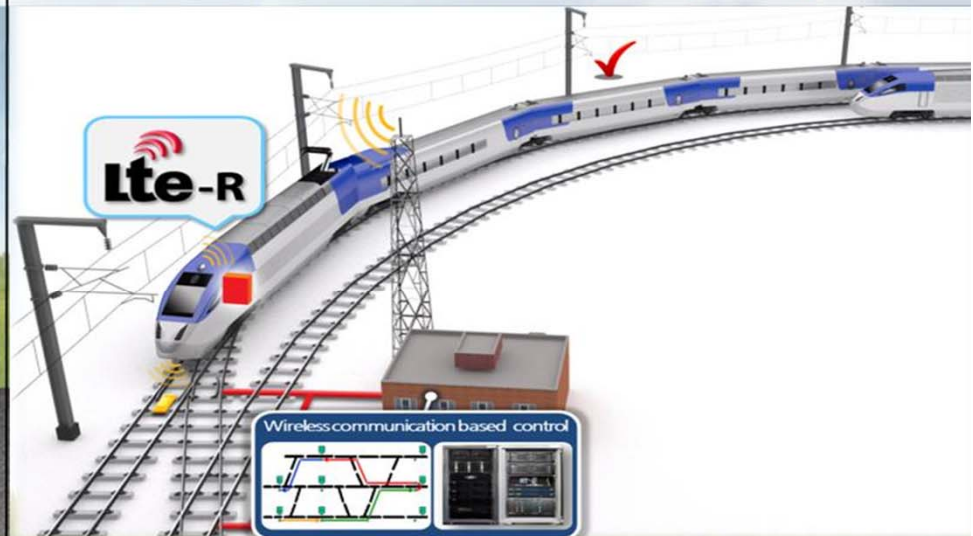
Train Control with LTE-R enables accurate train control in the high speed
