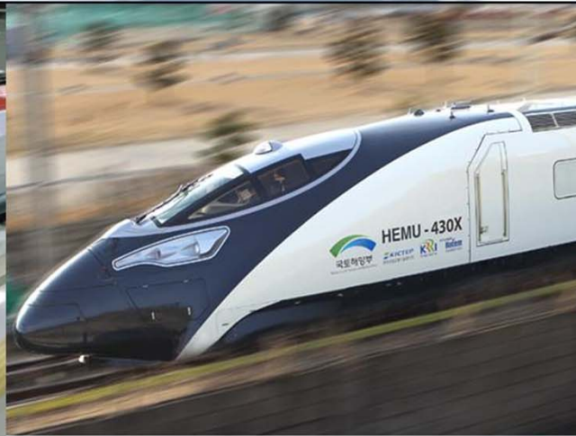
High Speed Train (430 km/h ) First Korea's electric multiple unit (4th speed record in the world)
