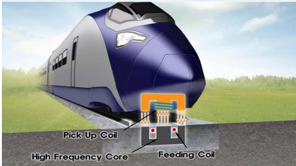
Wireless power transmission enables transmitting high power
