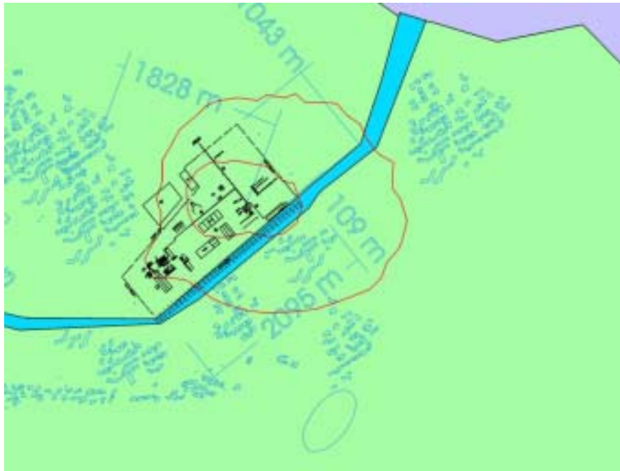
Figure 10. Discrepancy in the results of individual risk calculations relevant to risk-informed Land Use Planning: Maximum and minimum distances for the isorisk curve 10^{-5} \text{ yr}^{-1} (same figure as Figure 3)
