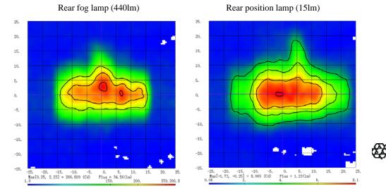
The simulation indicates that rear fog lamp has a maximum intensity of 266.8cd and rear position lamp has a maximum intensity of 8.1cd. According to the ratio of luminous flux of the two filaments, the maximum intensity of rear position lamp should be 9.1, but it is simulated to be 8.1. The reason is that the mail filament positioned and the second filament is not positioned on the focus of the reflector.
