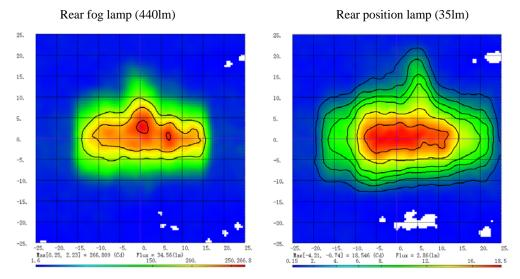
The simulation indicates that rear fog lamp has a maximum intensity of 266.8cd and rear position lamp has a maximum intensity of 18.5cd.
