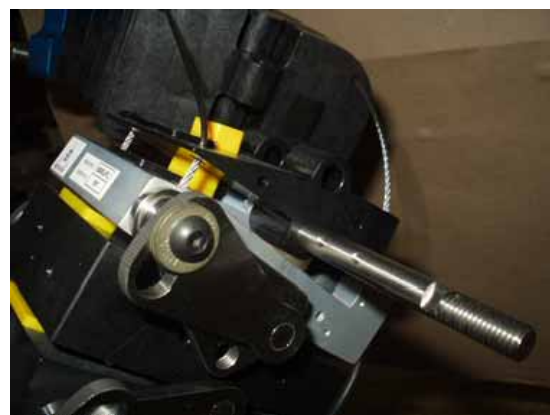
Figure 107 - Remove T1 Pin
