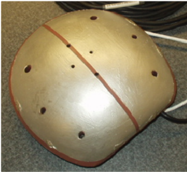
Figure 18 - Skull Cap Contact Switch
