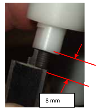
Figure 85 - Front and Rear Spring Adjustment if Back Angle cannot be Held
