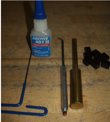
Figure 95 - Bumper Replacement Tools
