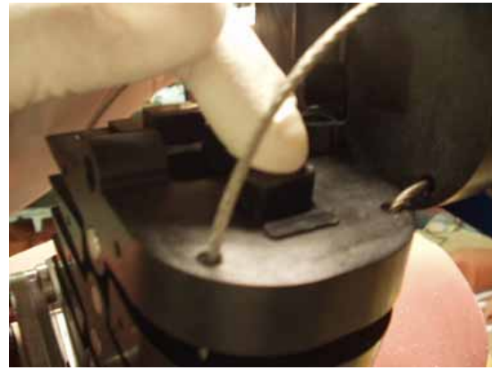
Figure 105 - Place in Bumper and Hold
