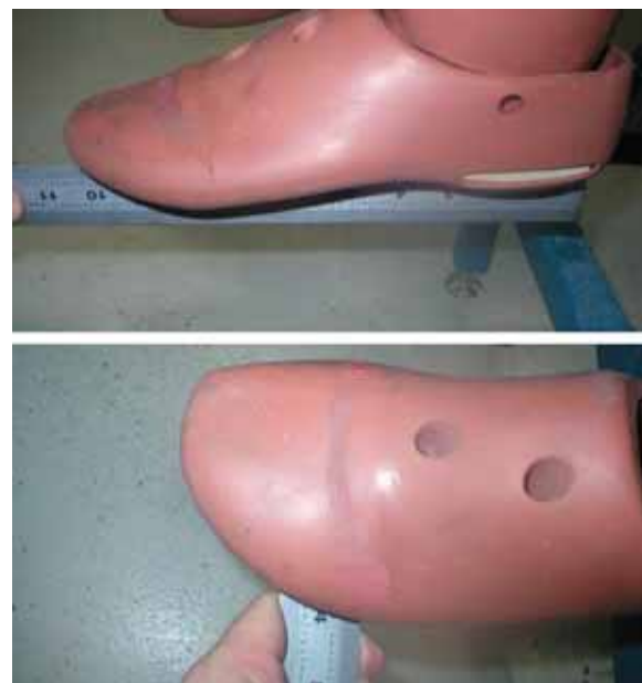
Figure 127 - Foot Length and Width
