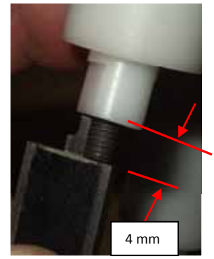
Figure 83 - Front and Rear Spring Adjustment if Front Angle cannot be Held
