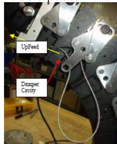
Figure 36 - Damper Cable Installation
