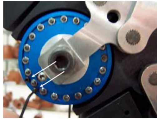
Figure 137 - Loosen M3 Clamping Screws
