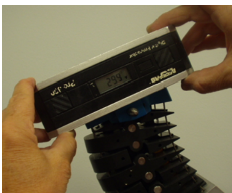
Figure 90 - OC Plate Angle Setting
