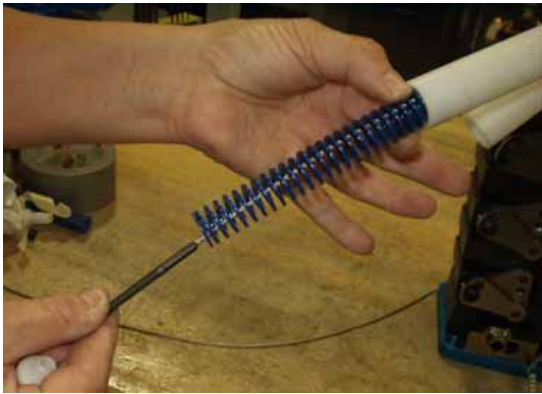
Figure 51- Anterior Spring Insertion
