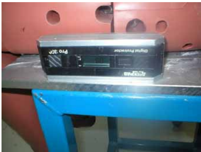
Figure 119 - Zero Angle Reference
