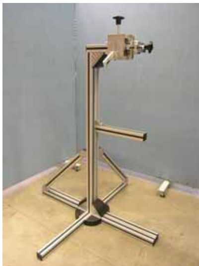
Fig. 6: Legform support rig for inverse tests
