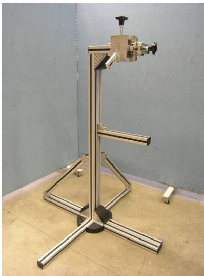
Fig. 8: Legform support rig for inverse tests
