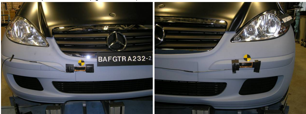
Figure 18 and 19: Two impact locations at the A-Class: Y = -232 mm and Y = 530 mm
