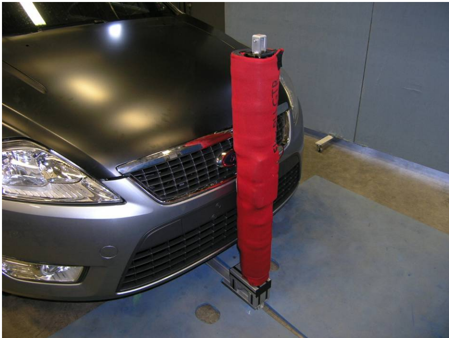
Fig. 12: Test setup for vehicle impacts
