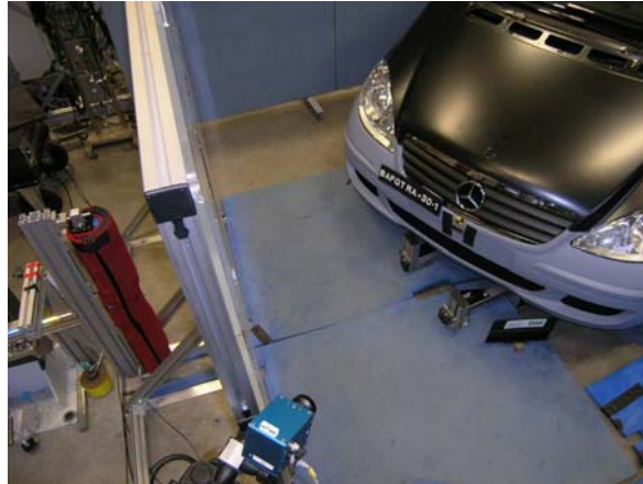
Fig. 20: Oblique vehicle test setup: +30°
