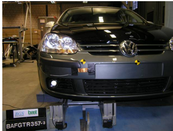
Figure 13: Two impact locations at the Golf: Y = 51 mm and Y = -357 mm
