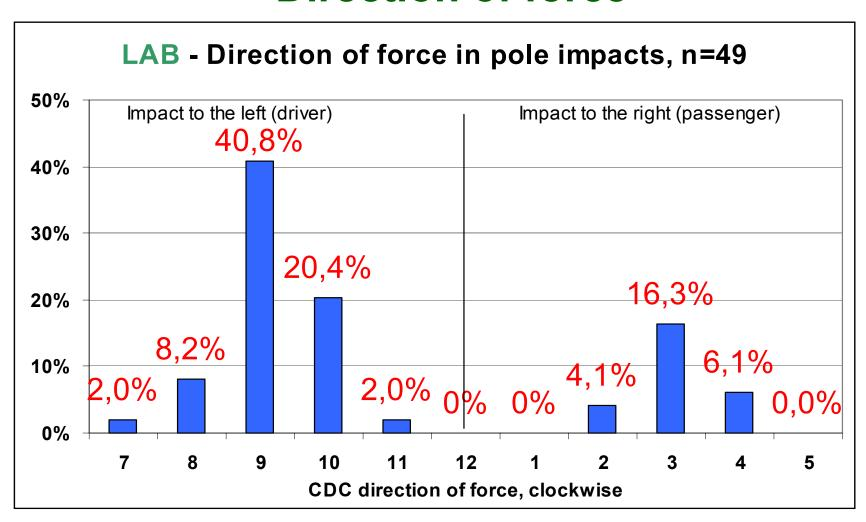
Result: Perpendicular is the most frequent impact direction
