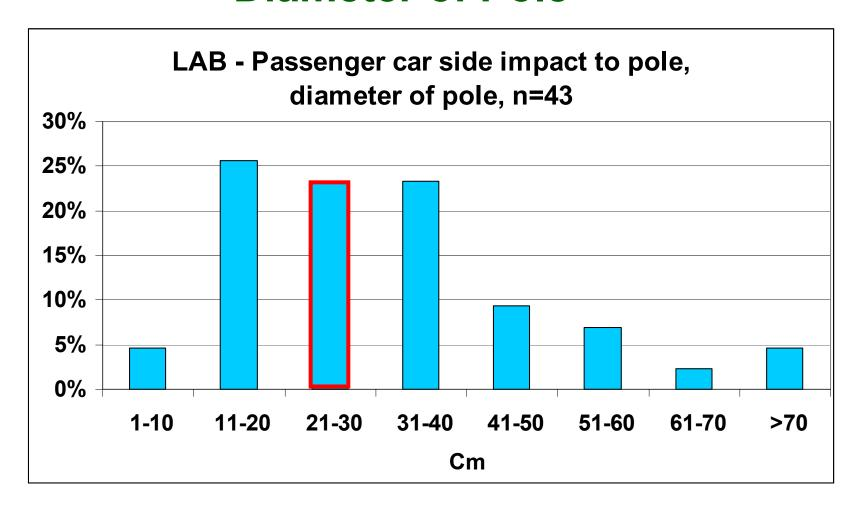
Result: The pole diameter in current tests seems appropriate
