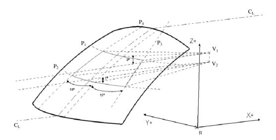
$C_L$ : trace of the longitudinal median plane of the vehicle
