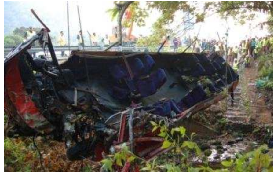
Damage on the bus structure.
