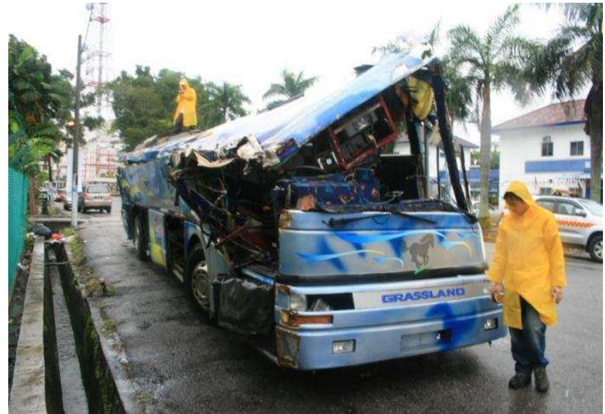
Damage on the bus structure.
