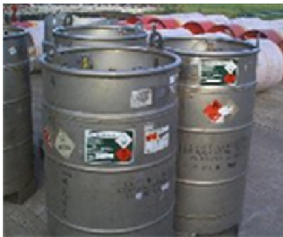
“pressure drum” = welded receptacle, between 150 L and 1000 L
