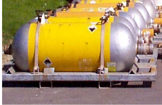
“tube”= seamless receptacle, between 150 L and 3000 L
