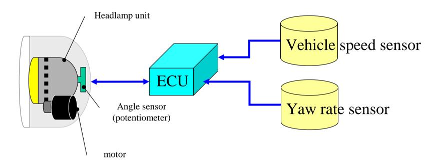
System construction diagram
