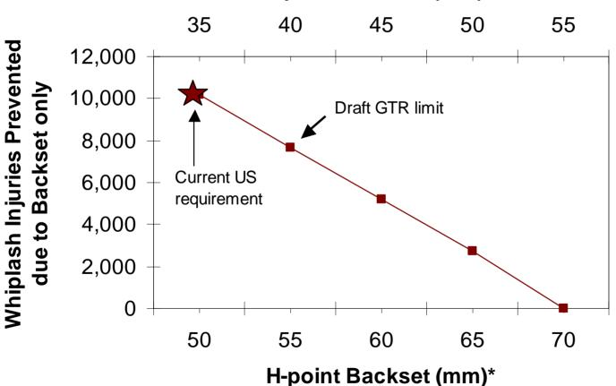
\*H-point value adjusted for seat back angle measured at manufacturers design angle
