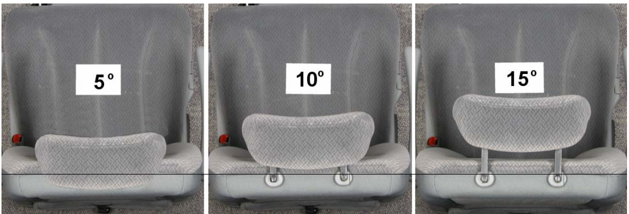
Figure 3. Top-view photos of the three head restraint conditions.
