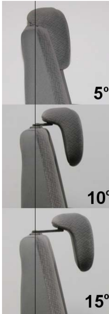
Figure 2. Side-view photos of the three head restraint conditions, stowed.
