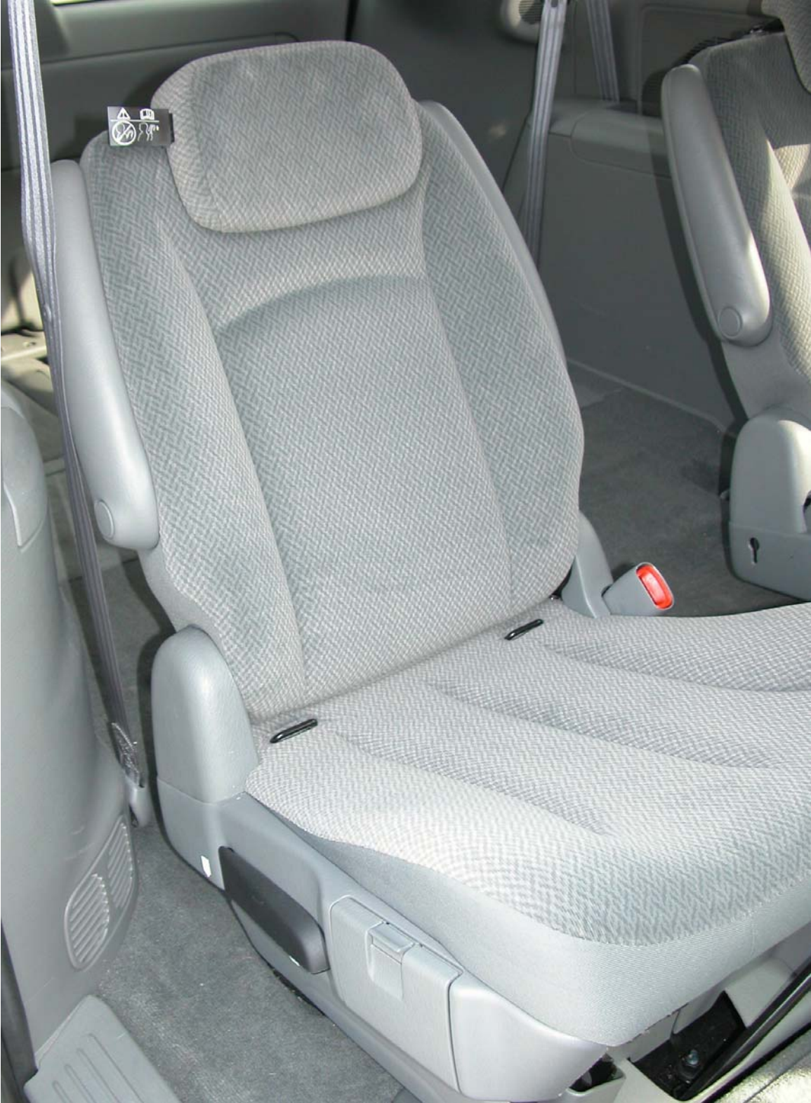
Figure 8. Modified head restraint label as mounted for testing.
