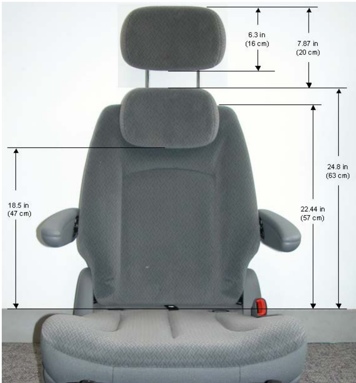
Figure 11. Approximate dimensions of second-row seat from a 2005 Chrysler Town and Country minivan (Note: photo was edited to show both stowed and fully extended positions of the head restraint).
