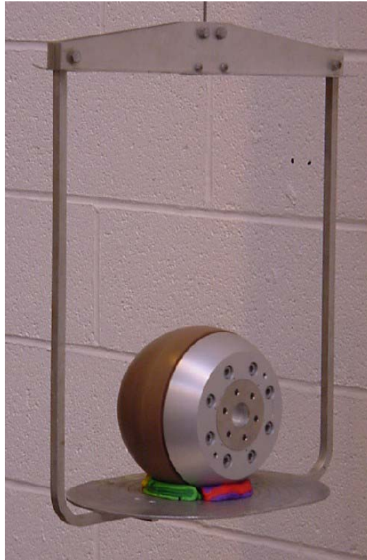
Figure 2.3. Headform on the torsion pendulum table with supporting plasticine
