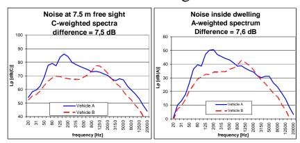
C-weighted spectrum on 7.5 meter is a good predictor for
