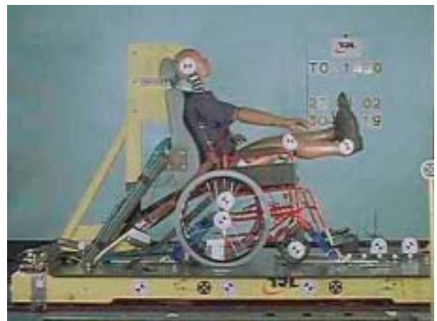
Figure 27b Wheelchair occupant with a gap between head and back restraint and occupant
