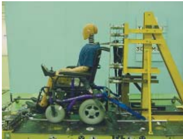
Figure 31 M3 rear facing – head and back restraint load
