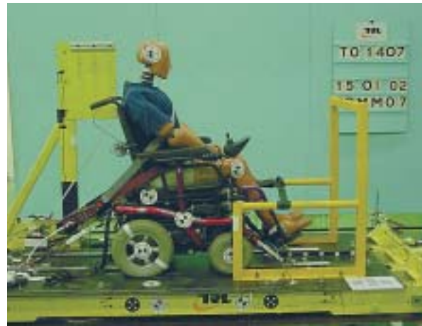
Figure 10 Set up with floor anchorage location for diagonal occupant restraint
