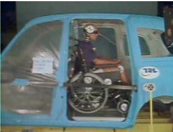
Figure 18a Set up with no head and back restraint
