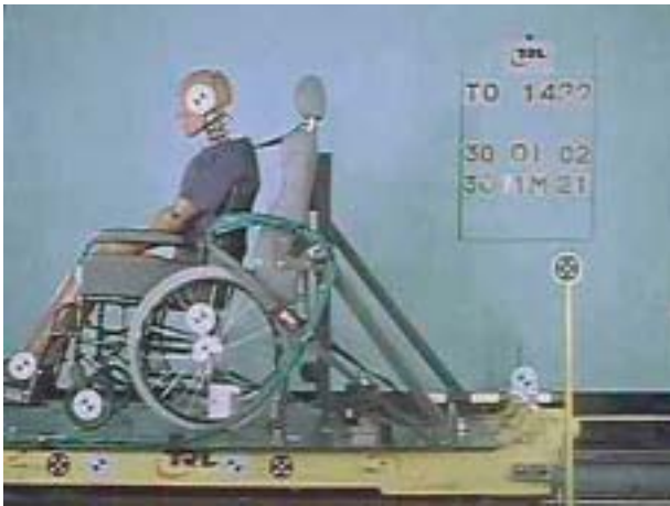
Figure 33a Set up with a gap between head and back restraint and occupant
