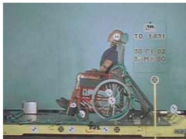
Figure 32b Wheelchair occupant with a head and back restraint
