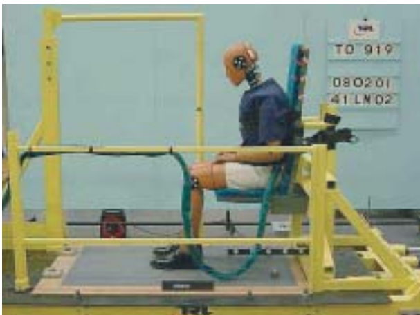
Figure 29 M3 rear facing – vehicle seated
