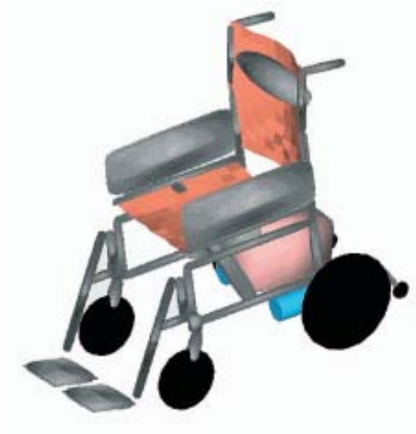
Figure C2 MADYMO model of the electric wheelchair
