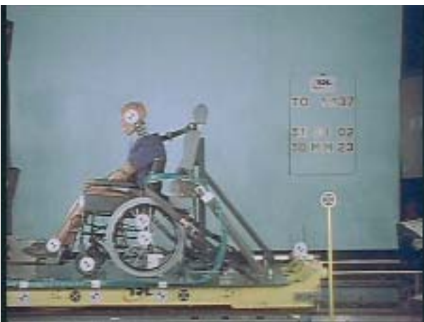
Figure 20a Set up with a gap between head and back restraint and occupant
