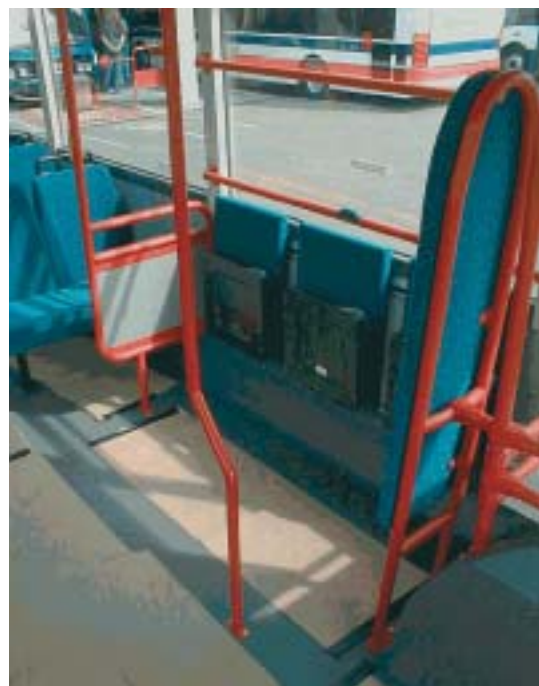
Figure 34 Wheelchair space in Optare Excel
