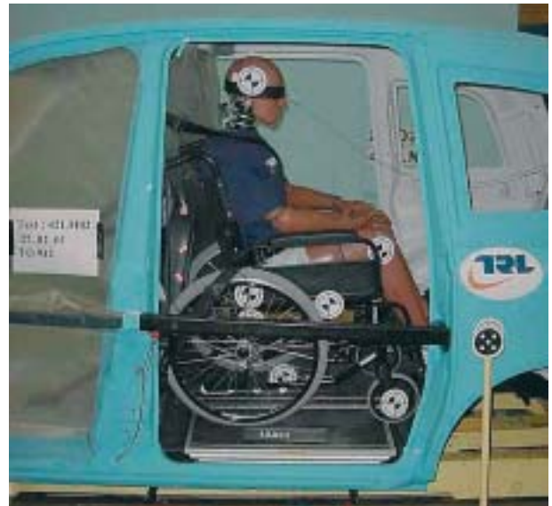
Figure 16 M1 and M2 rear facing – wheelchair seated
