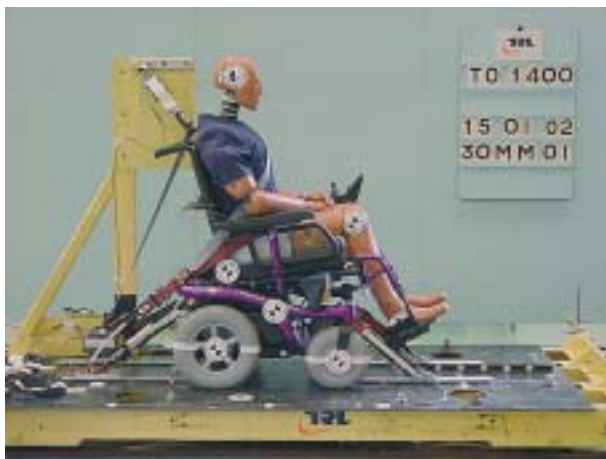
Figure 23 Set up with an upper location for the diagonal belt anchorage
