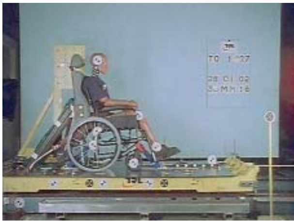
Figure 26a Set up with a head and back restraint
