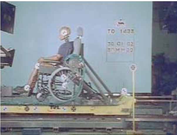
Figure 19a Set up with a head and back restraint
