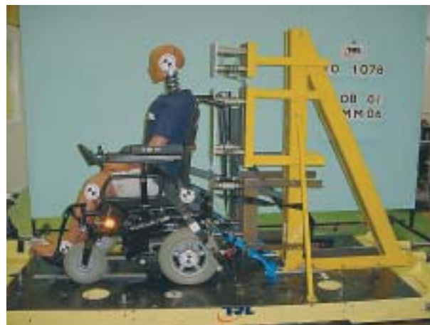
Figure 17 M1 and M2 rear facing – head and back restraint load
