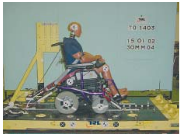
Figure 24 Set up with a floor location for the diagonal belt anchorage
