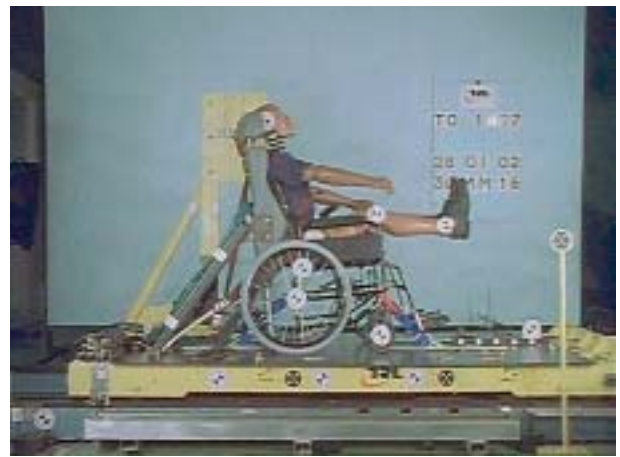
Figure 26b Wheelchair occupant with a head and back restraint
