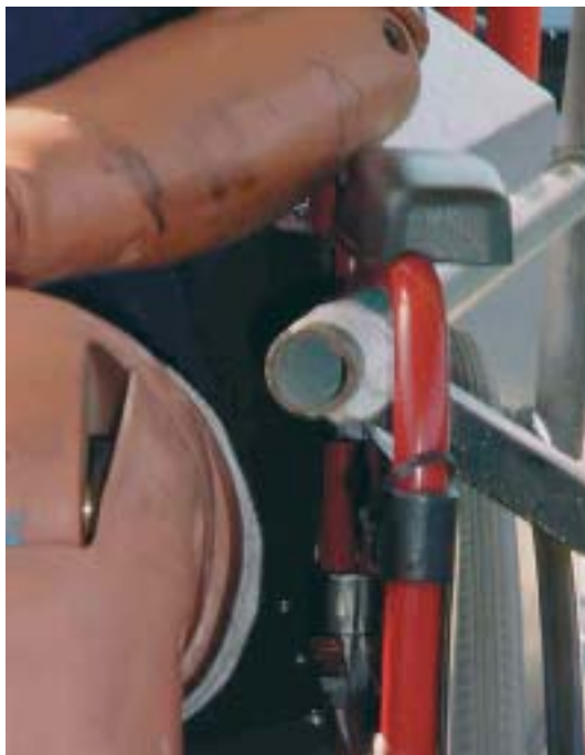
Figure 37 Post test with rail at 600 mm above floor
