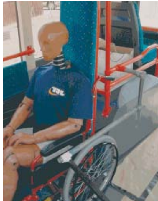
Figure 36 Wheelchair space fitted with rail
