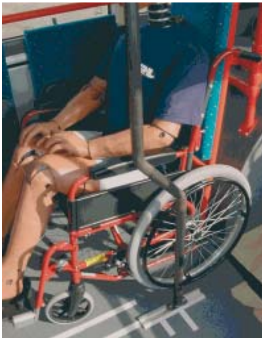
Figure 35 Wheelchair space fitted with stanchion
