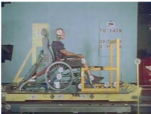
Figure 13a Set up with a gap between head and back restraint and occupant
