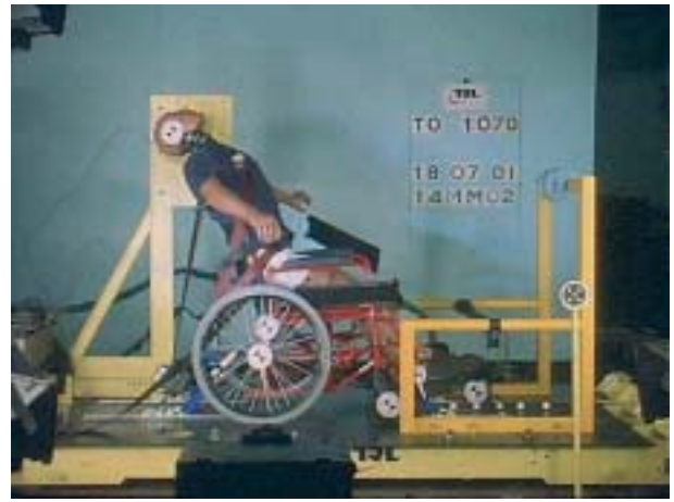
Figure 11b Wheelchair occupant with no head and back restraint
