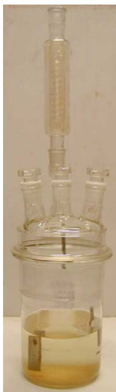
Figure 37.4.2: EXPOSURE RECEPTACLE WITH REFLUX CONDENSER
