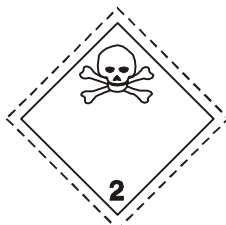
(No. 2.3) Toxic gases Symbol (skull and crossbones): black; Background: white; Figure '2' in bottom corner
